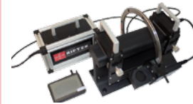
Rail Profile Measurement Gauge, PRP Series
