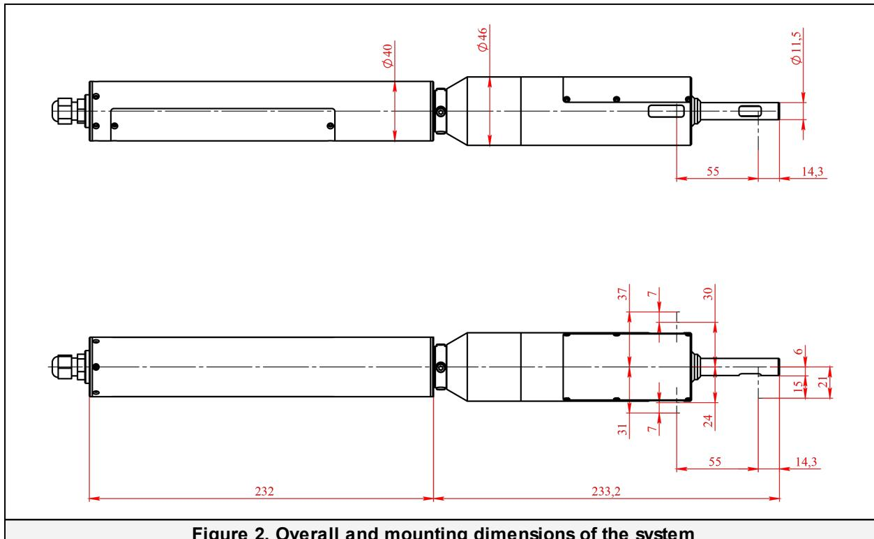
Figure 2. Overall and mounting dimensions of the system
