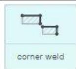
"corner weld" - угловой сварной шов:
