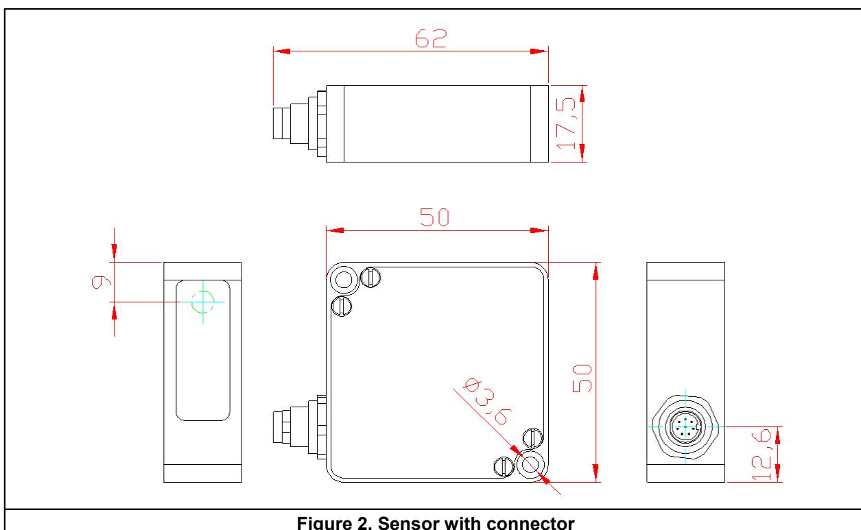
Figure 2. Sensor with connector
