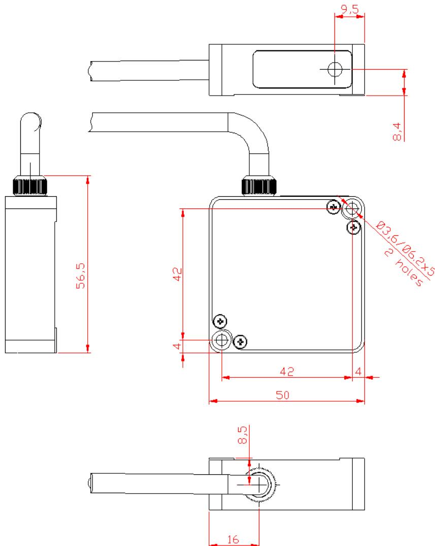
Figure 3. Sensor with cable gland
