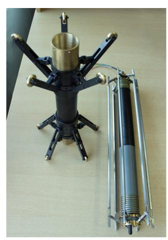
Centering frame is intended to hold measurement module near pipe axis for different pipe diameters.
