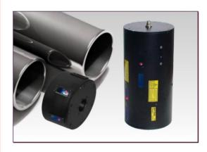
Systems are intended for contactless measuring of inner diameter and profiles of gun barrels, cylindrical and taper pipes, progressive cavity stators, turbodrills and so on.
