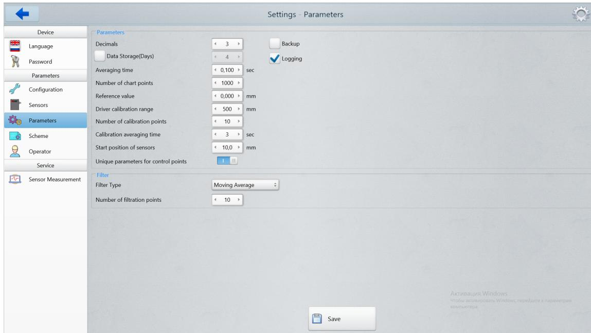
In the **Parameters** tab, the user can set general system parameters and filtering. The general parameters are described in the table below.
