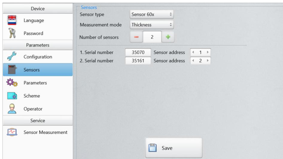
In the **Sensors** tab, the user can select the measurement mode, set the serial numbers of the sensors (when replacing) and their network addresses.
