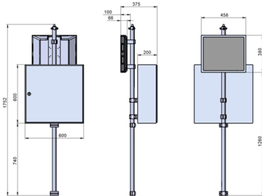
**Figure 4 - Overall and mounting dimensions of the control cabinet and panel computer**
