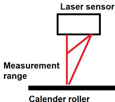
Since the laser sensor is calibrated in its own coordinate system, and thickness measurements are made in relation to the base surface (calender roller) on which the object is located, it is necessary to link the coordinates of the sensors and the base surface.
