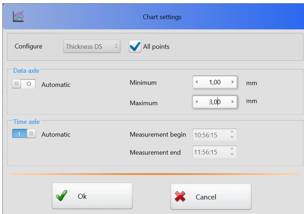
In the window that appears, you can configure the data or time axes to display data for all points or for each measurement point separately.
