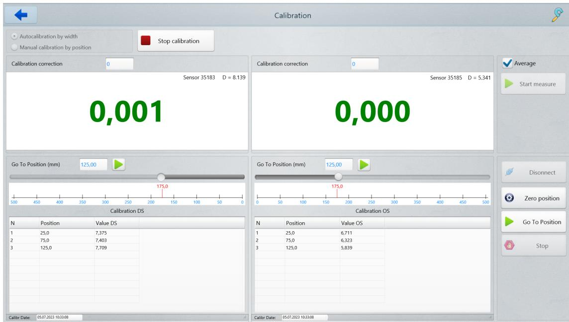
The system will begin calibrating along the entire length of the roller. During the calibration process, both sensors move sequentially to positions (10 default positions) evenly distributed along the roller and measure the distance to the roller. The measurement results are stored in the system memory and are used to calculate the thickness of the material.
