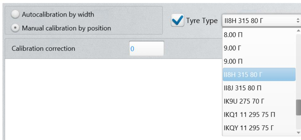
If a specific type of product is selected, the calibration position will be set automatically in accordance with the description of the measurement parameters for this type of material.
