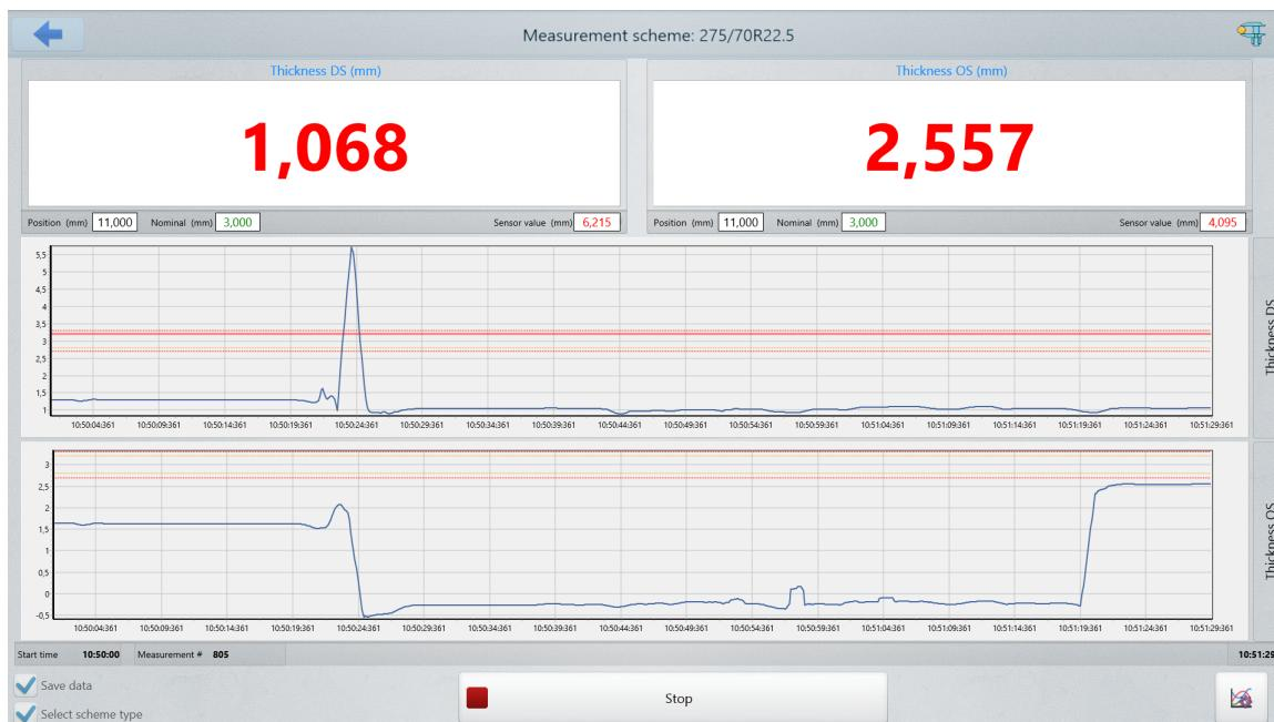
The measured thickness value at the control point, which is within the set tolerances, is displayed in green, outside the limits - in red.
