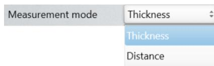
There are two measurement modes: **Thickness** and **Distance**.
